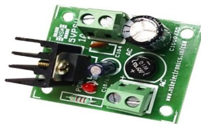
FIG 5: POWER SUPPLY UNIT
