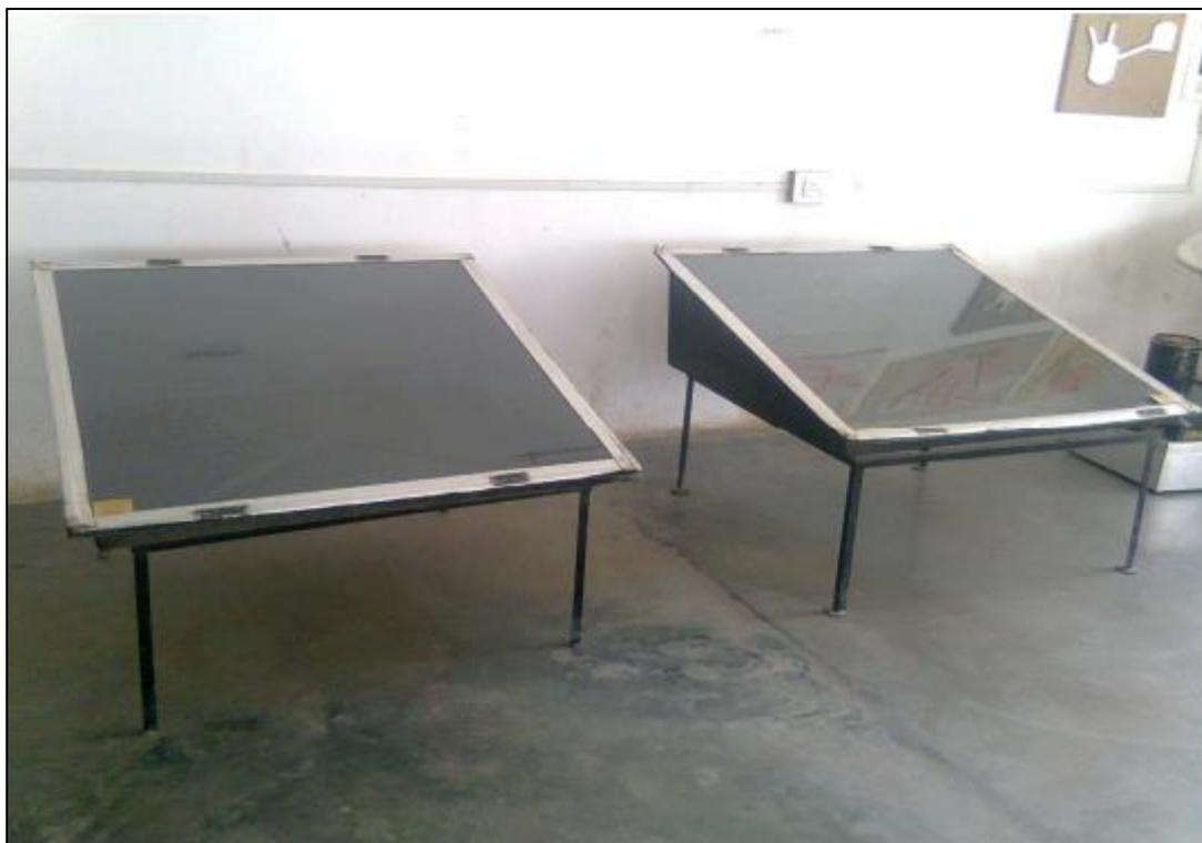
**Figure.1 Actual Single slope solar still**
