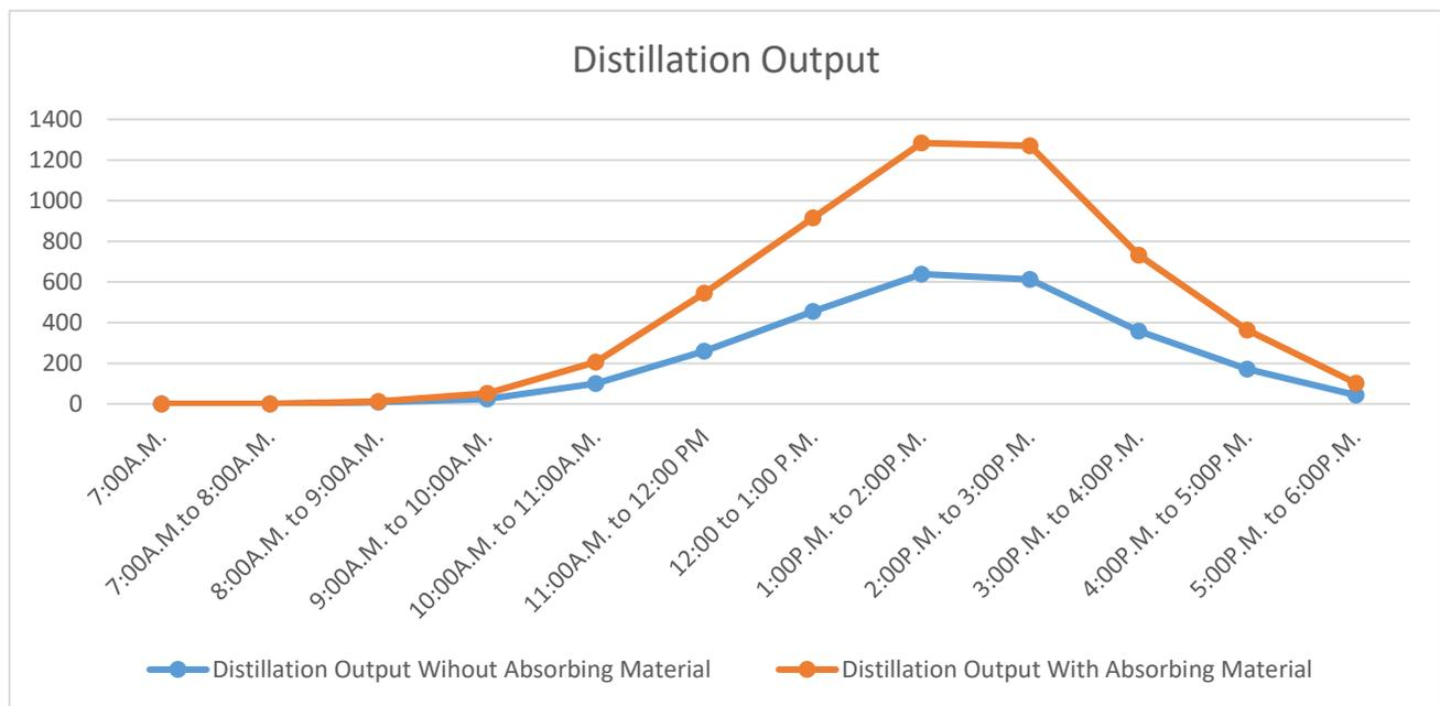
**Figure 4: productivity of solar still with and without included Aluminum foil.**
