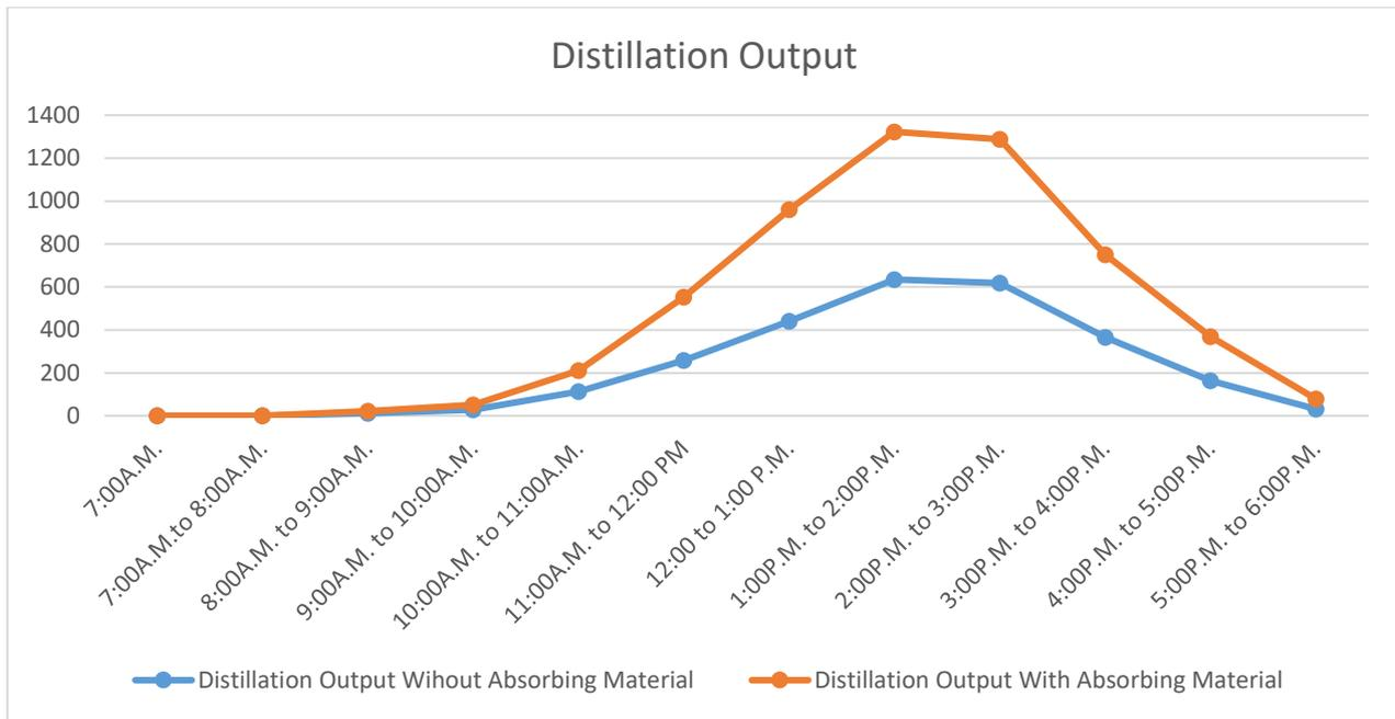
**Fig 2: productivity of solar still with and without included black brick particle**
