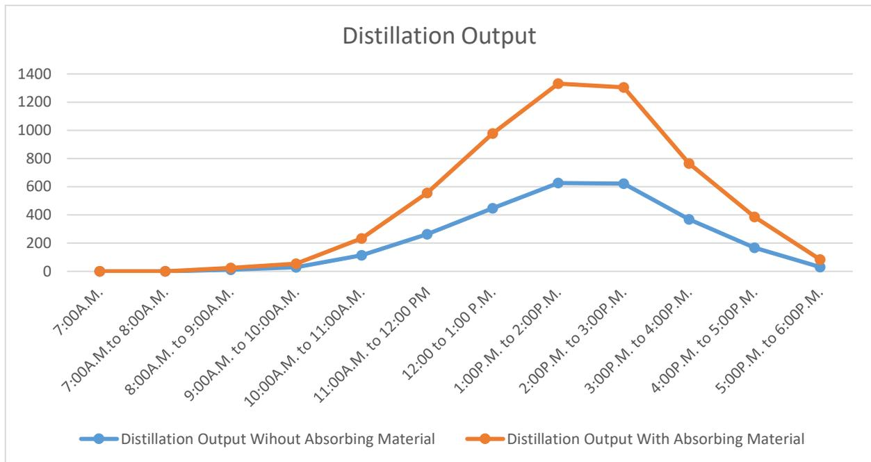
**Figure 3: productivity of solar still with and without included concreteparticle**
